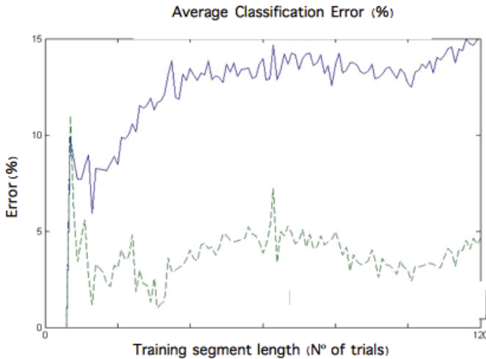
Fig. 13. SVM_OAO: ACE without PP (bold line) & after the 5 th PP step (dashed line)
